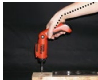
Pistol grip, ulnar deviation = bent wrist, poor wrist position
