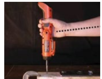
Inline grip, neutral = straight wrist, ideal wrist position
