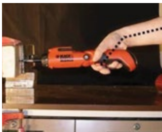
Inline grip, ulnar deviation = bent wrist, poor wrist position
