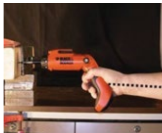
Pistol grip, neutral = straight wrist, ideal wrist position
